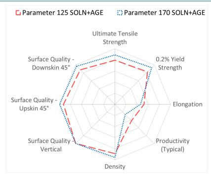
Spider Plot is generated by normalizing typical material data (containing both horizontal and vertical data) against a range defined for each material family. For **Maraging Steel** alloys, the ranges are as follows: UTS: 1650-2250 MPa, 0.2%YS: 1550-2150 MPa, Elongation: 0-10 %, Density: 99-100 %, Productivity: 5-30 cm<sup>3</sup>/h, Surface Quality (all): 40-5 µm
