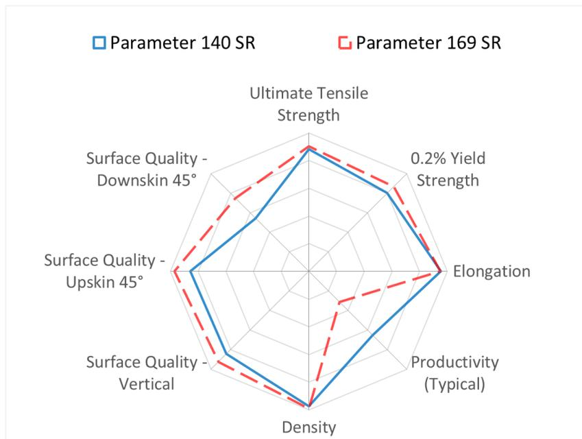
Spider Plot is generated by normalizing typical material data (containing both horizontal and vertical data) against a range defined for each material family. For nickel-based superalloy **Nickel 625**, the ranges are as follows: UTS: 0-1050 MPa, 0.2%YS: 0-750 MPa, Elongation: 0-50 %, Density: 99-100 %, Productivity: 5-30 cm<sup>3</sup>/h, Surface Quality (all): 40-5 µm
