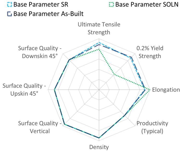
Spider Plot is generated by normalizing typical material data (containing both horizontal and vertical data) against a range defined for each material family. For **Stainless Steels**, the ranges are as follows: UTS: 0-750 MPa, 0.2%YS: 0-600 MPa, Elongation: 0-60 %, Density: 99-100 %, Productivity: 5-30 cm<sup>3</sup>/h, Surface Quality (all): 50-5 μm
