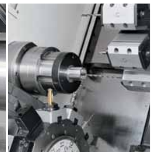
Increase work rigidity by PULL-Tension for Weak parts
