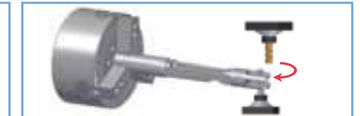
Increase work rigidity by PULL-Tension for Weak parts
