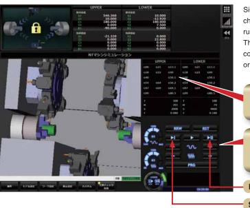
Simulation is performed to check the programs without running the machine.
