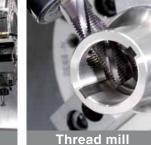
P1.5-INT Diameter :16mm :800min Cutting speed: 40m/min Machining Time: 55sec
