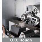
Diameter :65-45mm :1132min<sup>-1</sup> - 784min<sup>-1</sup> Feed :0.3mm/rev Cutting speed: 160m/min
