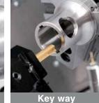
Wedge :32.5mm Length :N50-6814 Cutting speed :3m/min Machining Time: 84sec.
