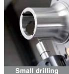
Type :0.5mm Diameter :6000min Feed :0.015mm/rev Cutting speed: 9.4m/min :3.5mm Machining Time: 25sec.
