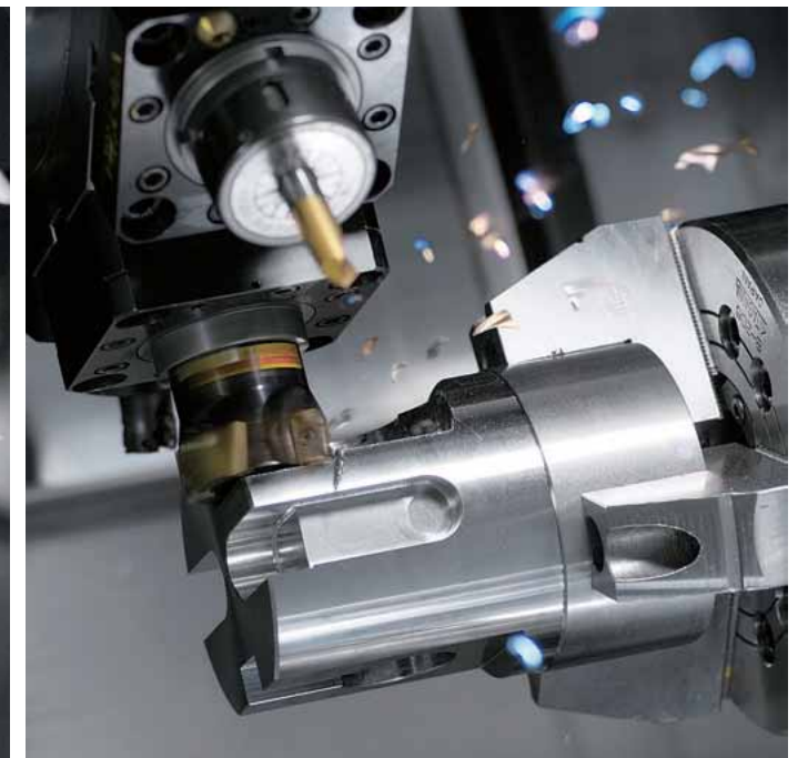
Dia. 50mm Face milling cutter Metal Removal Rate 148mL/min
