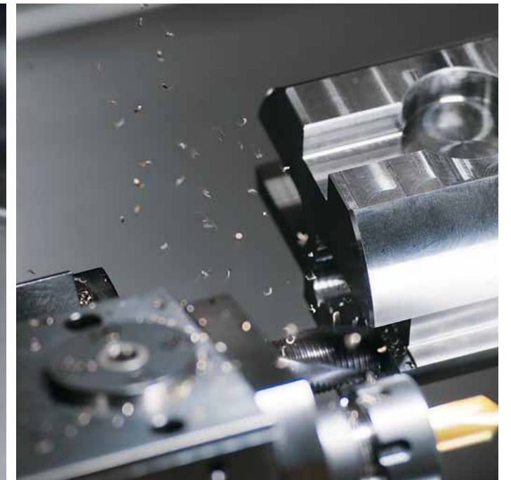
Dia. 20mm End mill Metal Removal Rate 34mL/min
