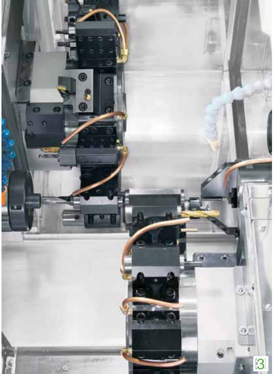
1 Upper-left/ lower-right turning operation 2 Upper-right/ lower-left operation 3 Upper-left/ lower-right operation
