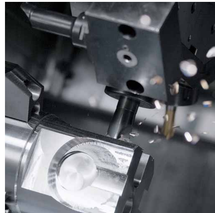
Dia. 25mm High feed end mill Metal Removal Rate 120mL/min
