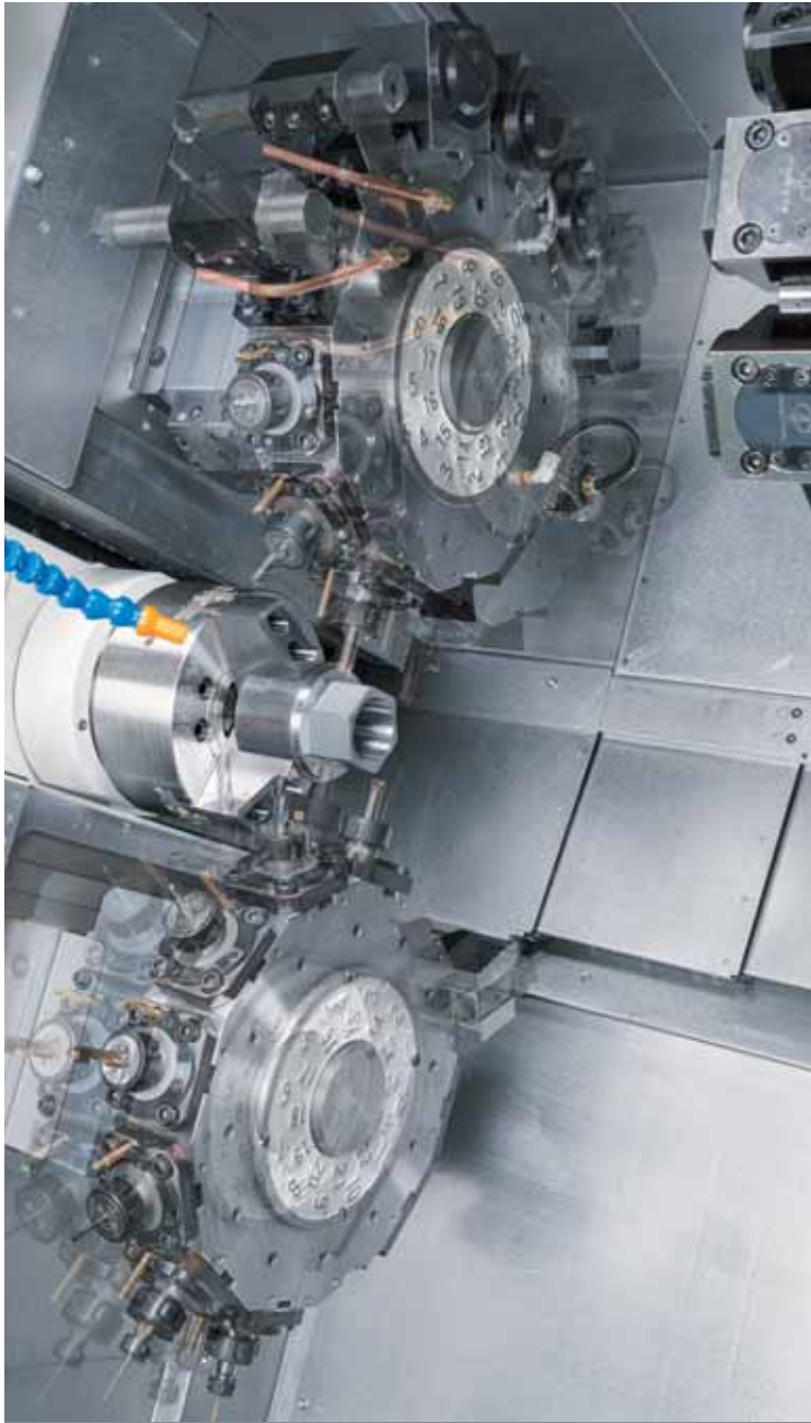
Simultaneous Milling with upper / lower tool on left spindle.
