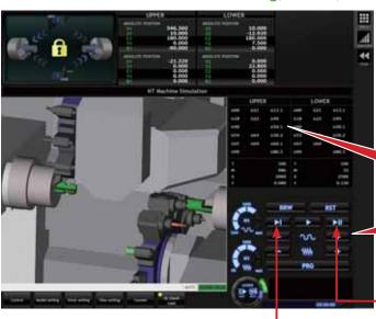
Simulation is performed to check the programs without running the machine.
