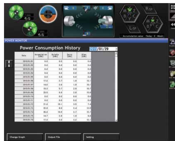
Power consumption history with numerical value. Spindle, Servo and Others are shown each day.
