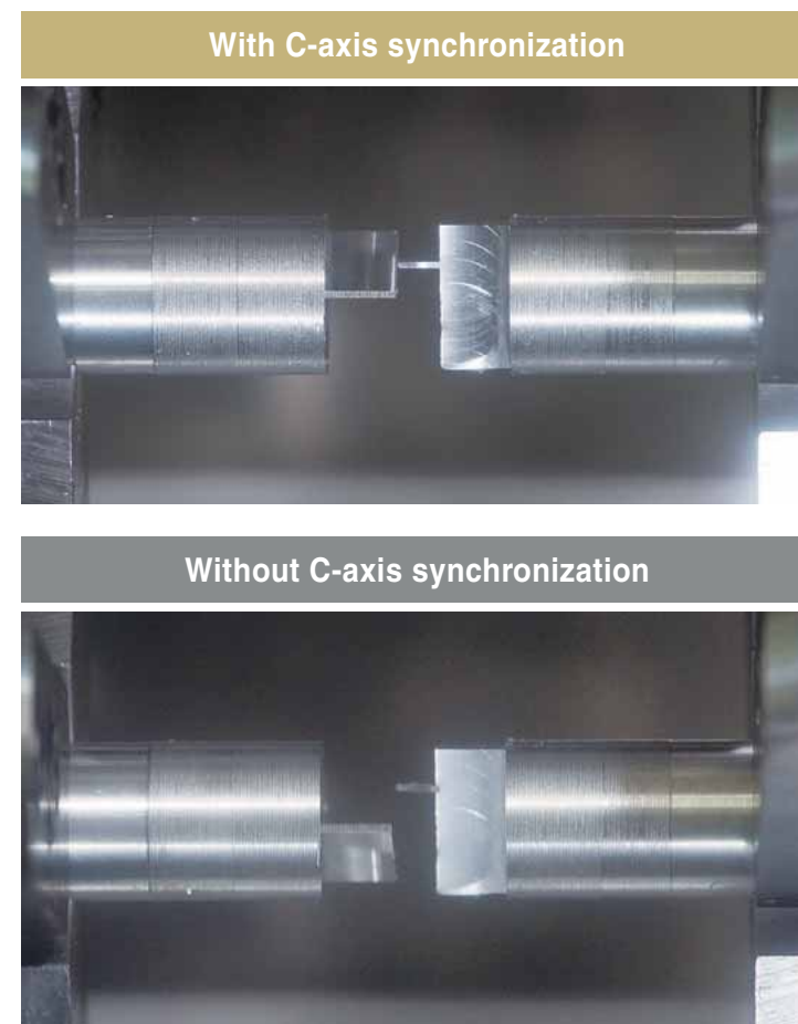
Picture 1 shows 1mm-thick rectangular segment in the middle. Picture 2 shows segment-fracture due to no C-axis synchronization
