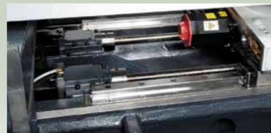
Z axis twin-ball-screw
